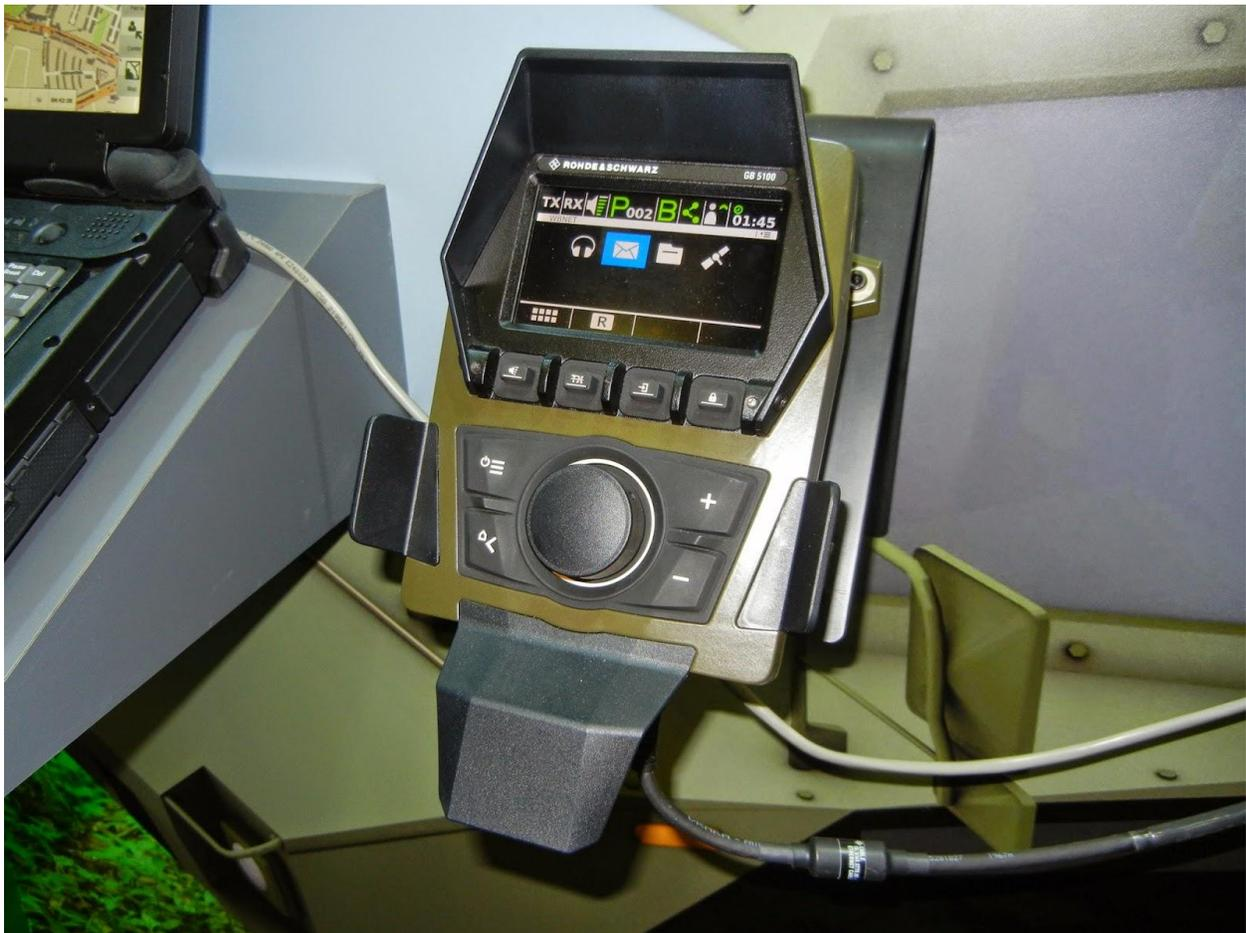
Vehicular radios have the ability to transmit and receive on everything they can listen to as long as they have a proper antenna installed for that band. All vehicles come with self tuning antenna systems but some of the Lower HF will have severely limited range if a longwire is not attached. The vehicular radios have multiple data interfaces and a dedicated computer and navigation database. These also contain an updateable atomic clock for a precision time base
