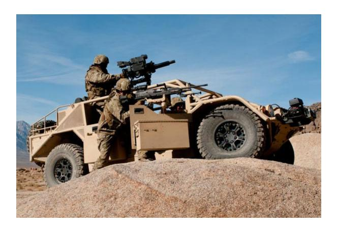
Morrow Industries advanced light strike vehicle (ALSV) is a lightweight, air transportable tactical wheeled vehicle designed and manufactured by Morrow Industries Defense for the US special operations command (SOCOM).
